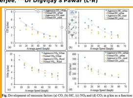
Development of emission factors (a) CO, (b) HC, (c) NOx and (d) CO2 in g/km as a function of speed.
